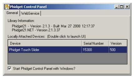
Double Click on the icon to activate the Phidget Control Panel and make sure that the **PhidgetLinearTouch** is properly attached to your PC.
