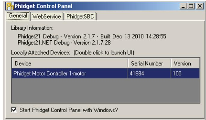
1. Double Click on **Phidget Motor Controller 1-Motor** in the Phidget Control Panel to bring up MotorControl-full and check that the box labelled Attached contains the word True.
