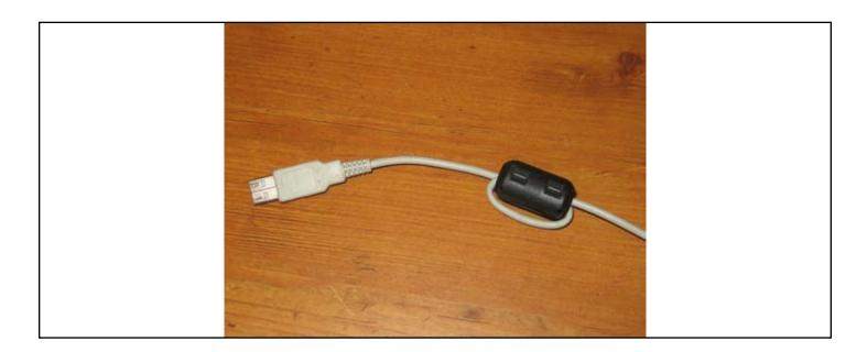
Our experimentation indicates that an extra loop through the ferrite bead is very helpful. Additional loops will often degrade protection. We suggest the ferrite bead shown above, as it is large enough to accommodate an extra loop of a USB cable, and can be easily snapped on or taken off. Digikey Part Number: 28A2736-OA2
